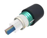
Fiber OSP cable, Steel Armored, Arid-Core, Dry Central Tube Ribbon, 24 fiber, Multimode OM4, bend insensitive, Feet jacket marking, Black jacket color
