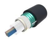
Fiber OSP cable, Steel Armored, Arid-Core, Dry Central Tube Ribbon, 72 fiber, Multimode OM3, bend insensitive, Feet jacket marking, Black jacket color
