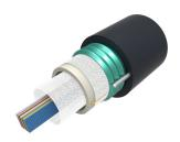
Fiber OSP cable, Steel Armored, Arid-Core, Dry Central Tube Ribbon, 12 fiber, Multimode OM3, bend insensitive, Feet jacket marking, Black jacket colorv
