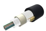
Fiber OSP Cable, Non-Armored, All-Dielectric, 192 fiber, Arid-Core, Dry Central Tube Ribbon, Multimode OM4 bend insensitive, Gel-free, Feet jacket marking, Black jacket color
