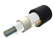
Fiber OSP Cable, Non-Armored, All-Dielectric, Arid-Core, 60 fibers, Dry Central Tube Ribbon, Multimode OM4 bend insensitive, Gel-free, Feet jacket marking, Black jacket color
