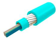
Fiber Indoor Cable, LSZH Riser, All-Dielectric, Central Tube Ribbon, Multimode, OM4, bend insensitive, 72 Fibers, Gel-free, Feet jacket marking, Aqua jacket color
