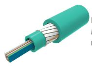
Fiber Indoor Cable, LSZH Riser, All-Dielectric, Central Tube Ribbon, Multimode, OM4, bend insensitive, 24 Fibers, Gel-free, Feet jacket marking, Aqua jacket color
