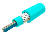
Fiber Indoor Cable, LSZH Riser, All-Dielectric, Central Tube Ribbon, Multimode, OM3, bend insensitive, 48 Fibers, Gel-free, Feet jacket marking, Aqua jacket color
