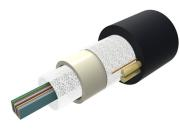
Fiber indoor/outdoor Cable, LSZH Riser All-Dielectric Central Tube Ribbon, Multimode OM4 bend insensitive, 24-fiber, feet jacket marking, black jacket color
