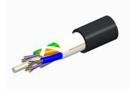
Fiber OSP cable, TeraSPEED® Single Jacket All-Dielectric, 144 fiber, Gel-Filled, Stranded Loose Tube, Composite OM3 and G.652.D and G.657.A1, Feet jacket marking, Black jacket color
