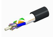
Fiber OSP cable, TeraSPEED® Single Jacket All-Dielectric, Gel-Free, 12 fibers, Stranded Loose Tube, Composite OM4 and G.652.D and G.657.A1, Feet jacket marking, Black jacket color
