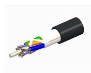
Fiber OSP cable, TeraSPEED® Single Jacket All-Dielectric, 108 fiber, Gel-Filled, Stranded Loose Tube, Composite OM3 and G.652.D and G.657.Al, Feet jacket marking, Black jacket color
