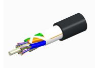
Fiber OSP cable, TeraSPEED® Single Jacket All-Dielectric, 12 fiber, Gel-Free, Outdoor Stranded Loose Tube w/HDPE Outer Jacket, Singlemode G.652.D and G.657.A1, Feet jacket marking, Black jacket color
