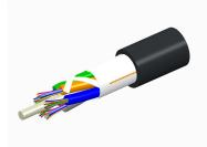
Fiber OSP cable, TeraSPEED® Single Jacket All-Dielectric, 144 fiber, Gel-Free, Outdoor Stranded Loose Tube w/HDPE Outer Jacket, Singlemode G.652.D and G.657.A1, Feet jacket marking, Black jacket color
