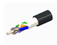
Fiber OSP cable, TeraSPEED® Single Jacket All-Dielectric, 72 fiber, Gel-Free, Outdoor Stranded Loose Tube w/HDPE Outer Jacket, Singlemode G.652.D and G.657.Al, Feet jacket marking, Black jacket color
