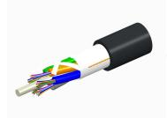
Fiber OSP cable, TeraSPEED® Single Jacket All-Dielectric, 24 fiber, Gel-Free, Outdoor Stranded Loose Tube w/HDPE Outer Jacket, Singlemode G.652.D and G.657.A1, Feet jacket marking, Black jacket color
