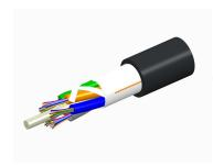
Fiber OSP cable, TeraSPEED® Single Jacket All-Dielectric, 12 fiber, Gel-Free, Outdoor Stranded Loose Tube w/HDPE Outer Jacket, Singlemode G.652.D and G.657.Al, Feet jacket marking, Black jacket color
