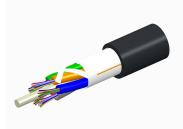
Fiber OSP cable, TeraSPEED® Single Jacket All-Dielectric, Gel-Free, 48 fibers, Stranded Loose Tube, Composite OM4 and G.652.D and G.657.A1, Feet jacket marking, Black jacket color
