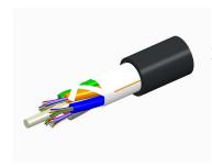
Fiber OSP cable, LazrSPEED® Single Jacket All-Dielectric, Gel-Free, Stranded Loose Tube, 24 fibers, Multimode OM3, Feet jacket marking, Black jacket color
