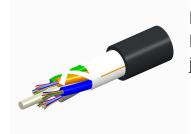
Fiber OSP cable, TeraSPEED® Single Jacket All-Dielectric, 132 fiber, Gel-Free, Stranded Loose Tube, Singlemode G.652.D and G.657.A1, Feet jacket marking, Black jacket color
