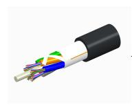
Fiber OSP cable, TeraSPEED® Single Jacket All-Dielectric, 196 fiber, Gel-Free, Stranded Loose Tube, Singlemode G.652.D and G.657.Al, Feet jacket marking, Black jacket color
