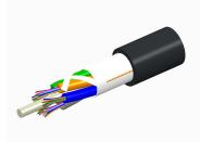
Fiber OSP cable, TeraSPEED® Single Jacket All-Dielectric, Gel-Free, Stranded Loose Tube, 12 fibers, Singlemode G.652.D and G.657.A1, Feet jacket marking, Black jacket color
