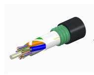
Fiber OSP cable, TeraSPEED® Single Jacket/Single Armor, 144 fiber, Gel-Free, Stranded Loose Tube, Singlemode G.652.D and G.657.Al, Meters jacket marking, Black jacket color
