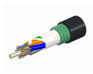
Fiber OSP cable, TeraSPEED® Single Jacket/Single Armor, Gel-Free, 6 fibers, Stranded Loose Tube, Singlemode G.652.D and G.657.A1, Meters jacket marking, Black jacket color
