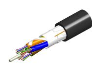
Fiber OSP cable, LazrSPEED®, Light Duty, Single Jacket, All-Dielectric, Gel-Free, Stranded Loose Tube, 2-fiber, Multimode OM4, Feet jacket marking, Black jacket color
