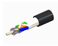
Fiber OSP cable, TeraSPEED® Single Jacket All-Dielectric, Gel-Free, Stranded Loose Tube, 18 fibers, Composite OM4 and G.652.D and G.657. Al, Feet jacket marking, Black jacket color
