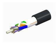
Fiber OSP cable, LazrSPEED® Single Jacket All-Dielectric, Gel-Free, Stranded Loose Tube, 24 fibers, Multimode OM4, Feet jacket marking, Black jacket color
