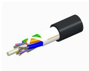
Fiber OSP cable, LazrSPEED® Single Jacket All-Dielectric, Gel-Free, 2 fiber, Stranded Loose Tube, Multimode OM4, Feet jacket marking, Black iacket color
