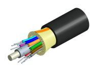
Fiber Indoor/Outdoor cable, TeraSPEED® Low Smoke Zero Halogen Riser Distribution, 18 fiber single-unit, Gel-free, Singlemode G.652.D and G.657.A1, Feet jacket marking, Black jacket color, Dca flame rating
