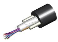
Fiber Indoor/Outdoor cable, Single Jacket Gel-Filled All-Dielectric, 36 fibers, Riser Rated Central Tube, Singlemode G.657.A2/B2, Feet jacket marking, Black jacket color
