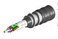
Fiber indoor/outdoor cable, LazrSPEED®, Plenum Rated, Gel-Free, Stranded Loose Tube with Aluminum Interlocking Armor containing a Plenum Rated Outer Jacket, 36 fiber, Multimode OM3, Feet jacket marking, Black jacket color
