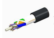
Fiber indoor/outdoor cable, LazrSPEED®, Single Jacket All-Dielectric, Low Smoke Zero Halogen (LSZH), 24 fiber, Gel-Free, Stranded Loose Tube, Multimode OM3, Black jacket color, Custom cable marking, Eca flame rating
