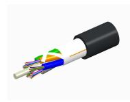
Fiber indoor/outdoor cable, TeraSPEED®, Single Jacket All-Dielectric, Low Smoke Zero Halogen (LSZH), 6 fiber, Singlemode G.652.D and G. 657.Al, Gel-Free, Stranded Loose Tube, Black jacket color, Custom cable marking, Eca flame rating
