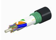
Fiber indoor/outdoor cable, LazrSPEED®, Single Jacket/Single Armor, Low Smoke Zero Halogen (LSZH), 48 fiber, Gel-Free, Stranded Loose Tube, Multimode OM3, Black jacket color, Feet jacket marking
