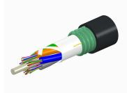
Fiber indoor/outdoor cable, TeraSPEED®, Single Jacket/Single Armor, Low Smoke Zero Halogen (LSZH), 6 fiber, Singlemode G.652.D and G. 657.A1, Gel-Free, Stranded Loose Tube, Black jacket color, Feet jacket marking
