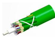
Fiber indoor cable, TeraSPEED® Plenum Distribution, 36 fiber multi-unit with 12 fiber subunits, Singlemode G.652.D and G.657.A1, Gel-free, Feet jacket marking, Green jacket color
