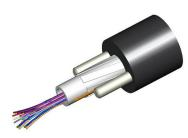
Fiber indoor/outdoor, TeraSPEED® Single Jacket Gel-Filled All-Dielectric Riser Rated Central Tube, 12 fibers, Singlemode G.652.D and G.657.Al, Feet jacket marking, black jacket color
