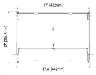
The overall width of the panels, including the mounting brackets, is 19" [482.6mm] or 23" [584.2mm] depending on which brackets are installed. The height of the panels can be found in this table:
