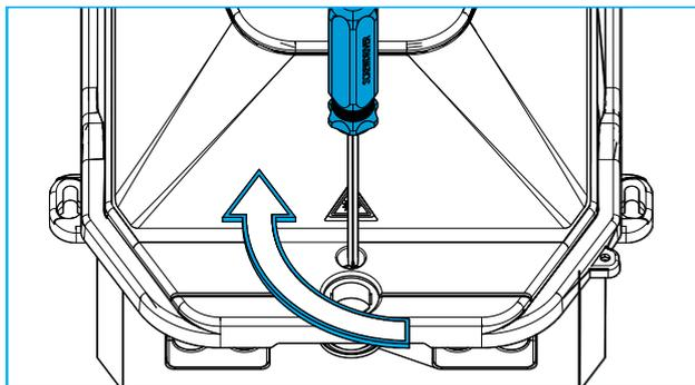
1 Secure by turning the locking screw.
