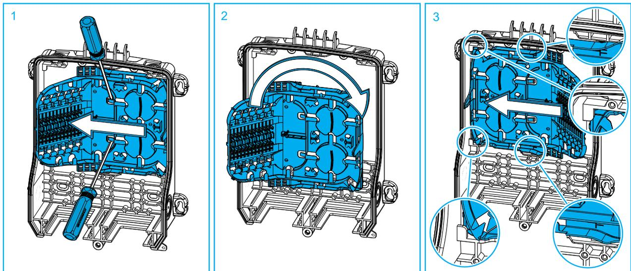
1 Use a screwdriver to elevate the locking lips and push the organizer to the side to release.
