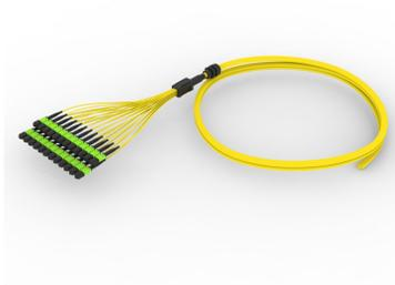
Ultra Low Loss Method A Singlemode MPO16 Pinned to Unconnectorized Pre-terminated Trunk Cable, 288-Fiber, Low Smoke Zero Halogen/Riser, 200µm 16F Rollable Ribbon
