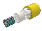
Fiber indoor cable, All-Dielectric, LSZH/Riser-Rated, Gel-Free, Central Tube 200µm Rollable Ribbon, 144 fiber, Singlemode G.657.A2/B2, Feet jacket marking, Yellow jacket color, Cca flame rating
