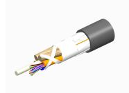
Fiber indoor/outdoor cable, LazrSPEED®, Single Jacket All-Dielectric, Plenum Rated, Multimode OM4, Gel-Free, 36 fiber, Stranded Loose Tube, PVDF jacket, Black jacket color, Feet cable marking
