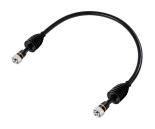
HELIAX® 1/2" Superflexible Fire retardant SureFlex® Jumper with interface types 4.3-10 Male and 4.3-10 Male, 1M with black non-halogenated fire-retardant polyolefin jacket. with HELIAX® SureGuard weatherproofing
