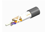
Fiber indoor/outdoor cable, LazrSPEED®, Single Jacket All-Dielectric, Plenum Rated, Gel-Free, 144 fiber, Stranded Loose Tube, PVDF jacket, Multimode OM3, Black jacket color, Feet cable marking
