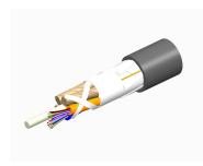
Fiber indoor/outdoor cable, LazrSPEED®, Single Jacket All-Dielectric, Plenum Rated, Gel-Free, Stranded Loose Tube, PVDF jacket, 72 fiber, Multimode OM3, Black jacket color, Feet cable marking
