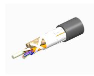
Fiber indoor/outdoor cable, TeraSPEED®, Single Jacket All-Dielectric, Plenum Rated, 48 fiber, Singlemode G.652.D and G.657.Al, Gel-Free, Stranded Loose Tube, PVDF jacket, Black jacket color, Feet cable marking
