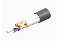
Fiber indoor/outdoor cable, LazrSPEED®, Single Jacket All-Dielectric, Plenum Rated, Gel-Free, 24 fiber, Stranded Loose Tube, PVDF jacket, Multimode OM3, Black jacket color, Feet cable marking
