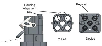
Align the M-LOC connector with the antenna mating interface and push firmly into place, eliminating gap between connector housing and bulkhead. While mating, a slight back and forth motion on the housing/cables will assist in centering and seating the port connectors into alignment. **Do Not** twist the jumpers. Push the latch toward the base of the antenna to engage the latch pins at the base of the connector housing.
