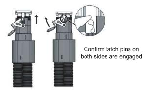
Apply force on the bent flange of the latch until the detents in the arms pop over the pins. There will be an audible and tactile click. To reduce hand strain, a screwdriver may be used.
