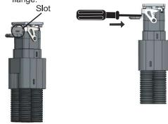
Grasp M-LOC connector housing, hold bent flange portion of latch back toward cable strain relief, pull the connector away from device. A slight back and forth motion on the housing helps to release the port connectors.
