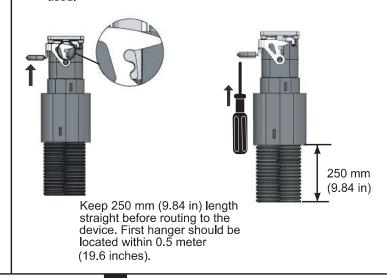
To remove the M-LOC connector pull latch flange away from the base of the antenna. To reduce hand strain, a flat blade screwdriver may be inserted in the slot above the latch flange and pulled down against the flange.
