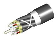
Fiber Indoor/Outdoor cable, TeraSPEED® Low Smoke Zero Halogen Riser Distribution, 48 fiber multi-unit with 12 fiber subunits, Gel-free, Singlemode G.652.D and G.657.A1, Feet jacket marking, Black jacket color, Cca flame rating
