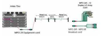
Figure 16: 120G parallel support with MPO-24
