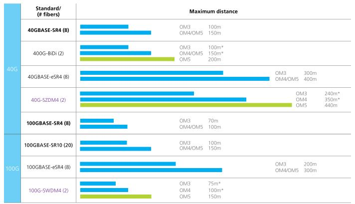
Figure 2: Ethernet network optic application - \* OM3/OM4 effective modal bandwidth is only specified at 850nm
